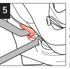
Thread the shoulder belt through the lock-off on the opposite side of the vehicle buckle. Close the lock-off. Lock by lifting up the tab to the locked position.
